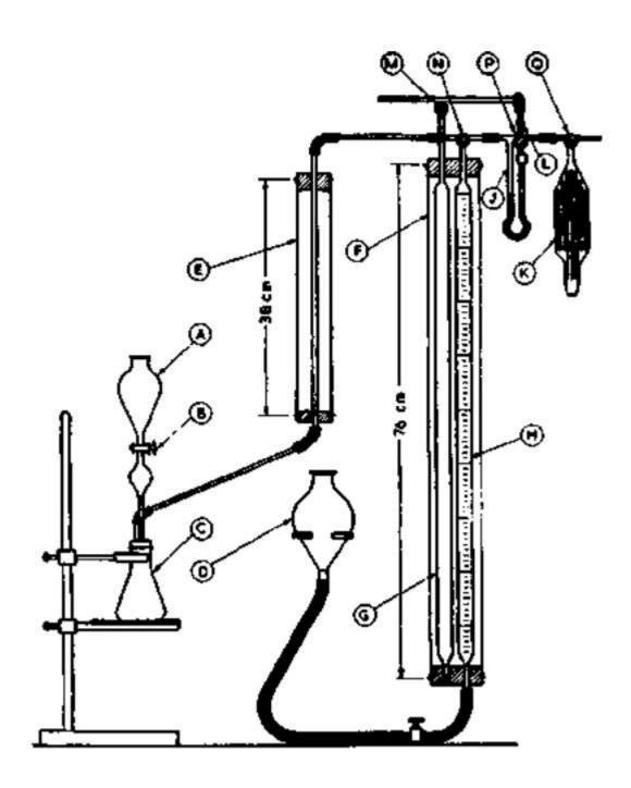
FIG. 1 ASSEMBLY OF APPARATUS FOR DETERMINATION OF CARBONATE
